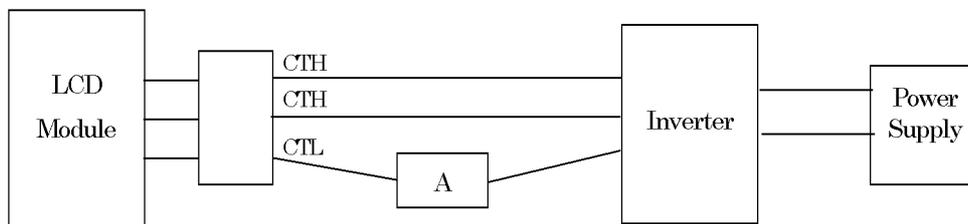
\*3) Lamp frequency of inverter may produce interference with horizontal synchronous frequency, and this may cause horizontal beat on the display. Therefore, please adjust lamp frequency, and keep inverter as far from module as possible or use electronic shielding between inverter and module to avoid the interference.
