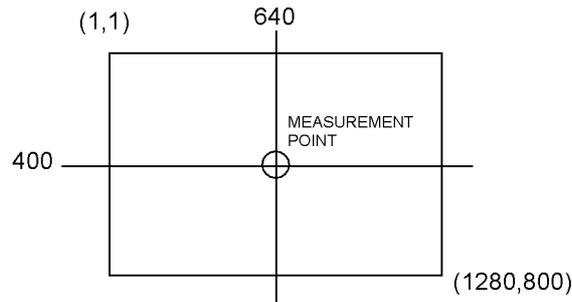
These items are measured when lamp units are assembled into T-55312D121J-FW-A-ABN, and using CS1000(MINOLTA) for color coordinates, and CS1000 or BM-5A(TOPCON) for Luminance under the dark room condition (no ambient light) after more than 30 minutes from turning on the lamp unless noted.
