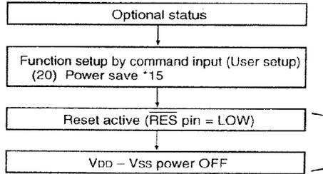
Set the time (t<sub>L</sub>) from reset active to turning off the V<sub>DD</sub> - V<sub>SS</sub> power (V<sub>DD</sub> - V<sub>SS</sub> = 1.8 V) longer than the time (t<sub>H</sub>) when the potential of V<sub>5</sub> - V<sub>1</sub> becomes below the threshold voltage (approximately 1 V) of the LCD panel. For t<sub>H</sub>, refer to the <Reference Data> of this event. When t<sub>H</sub> is too long, insert a resistor between V<sub>5</sub> and V<sub>DD</sub> to reduce it.
