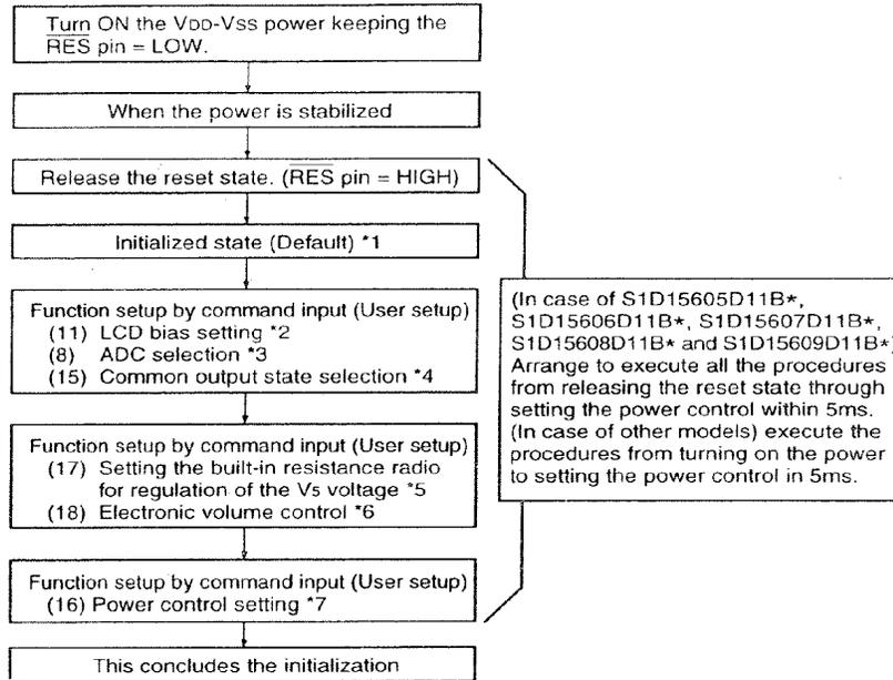
② When the built-in power is not being used immediately after turning on the power:
