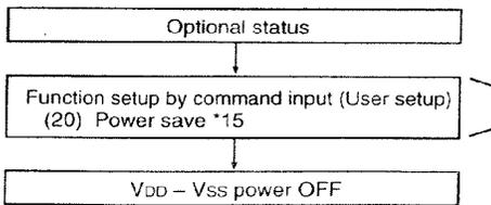
Set the time (t<sub>L</sub>) from power save to turning off the V<sub>DD</sub> - V<sub>SS</sub> power (V<sub>DD</sub> - V<sub>SS</sub> = 1.8 V) longer than the time (t<sub>H</sub>) when the potential of V<sub>5</sub> - V<sub>1</sub> becomes below the threshold voltage (approximately 1V) of the LCD panel.
