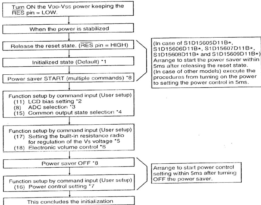
\* The target time of 5ms will result to vary depending on the panel characteristics and the capacitance of the smoothing capacitor. Therefore, we suggest you to conduct an operation check using the actual equipment.
