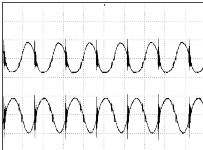
Figure 14: Output voltage ripple at nominal input voltage ( V_{in}=48V ) and rated load current ( I_{o1}=I_{o2}=2.7A ) (20 mV/div). Load capacitance: 1\mu F ceramic capacitor and 10\mu F tantalum capacitor. Bandwidth: 20 MHz. (See Figure 12). Scope measurement should be made using a BNC cable (length short than 20 inch). Position the load between 51 mm and 76 mm (2inch and 3 inch) from the module.
