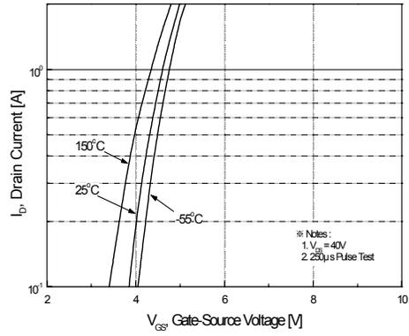
Figure 2. Transfer Characteristics
