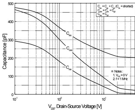
Figure 5. Capacitance Characteristics
