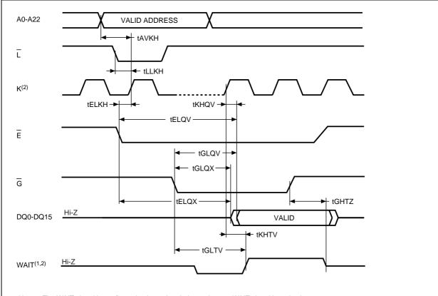
Note 1. The WAIT signal is configured to be active during wait state. WAIT signal is active Low.
