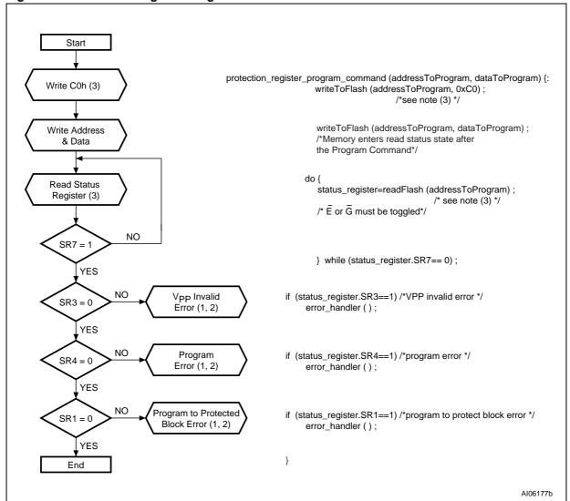
Figure 25. Buffer Enhanced Factory Program Flowchart and Pseudo Code
