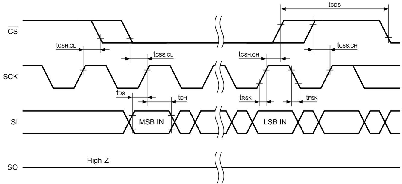
Figure 5 Serial Input Timing
