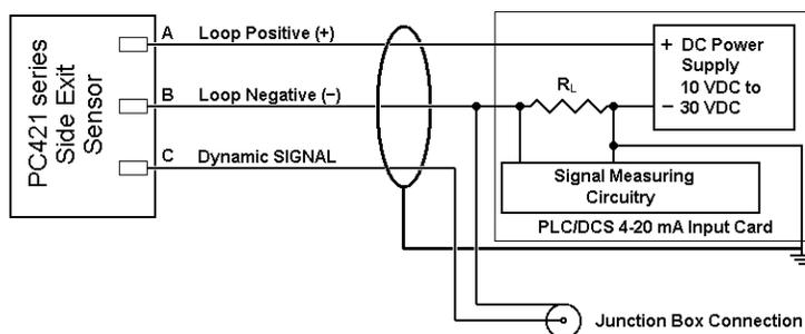
All wire and cable used for installation of PC421 series sensors should be shielded. Generally accepted instrumentation wiring practice considers the best way to ground the shield is to connect it at the measurement end of the cable. The shield should not be wired to ground at the sensor end of the cable. Wilcoxon R6W, R6GQAI, R6GQI and R6QI type connectors all leave the shield unconnected at the sensor end of the cable.
