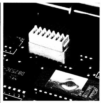
The NR connector is our first insulation displacement connector designed for printed circuit boards and has a justified reputation for reliability. The receptacle is color-coded according to the applicable wise size (AWG #28 green, AWG #26 white and AWG #24 black) and accepts both discrete wires and ribbon cables.
