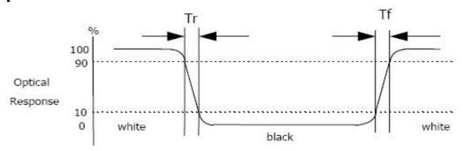
Response time is the time required for the display to transition from white to black (Rising time,  $T_r$ ) and from black to white (Falling time,  $T_f$ ) for additional information.
