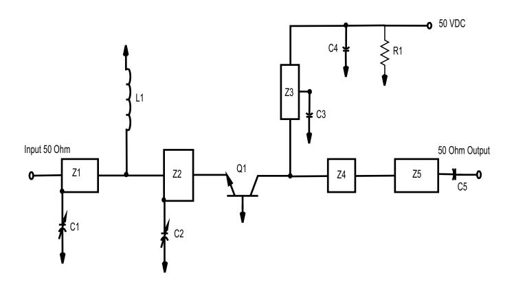
PC Board Material .010" Dielectric Teflon Fiberglass
