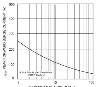
NUMBER OF CYCLES AT 60 Hz Fig. 3 Maximum Non-Repetitive Peak Forward Surge Current
