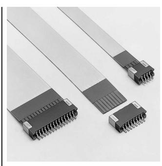
The FMS series connectors are designed for surface mounting (SMT) and to meet the demand for high-density packaging. They are miniature connectors with a height of only 2.8mm (.110"), and can be supplied packaged in embossed tape to facilitate automatic mounting.
