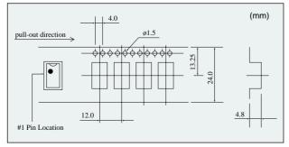
1,000 pieces/reel are boxed and shipped with the taping method as shown above
