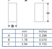
Soldering temperature should be 260°C for a maximum of 10 seconds.
