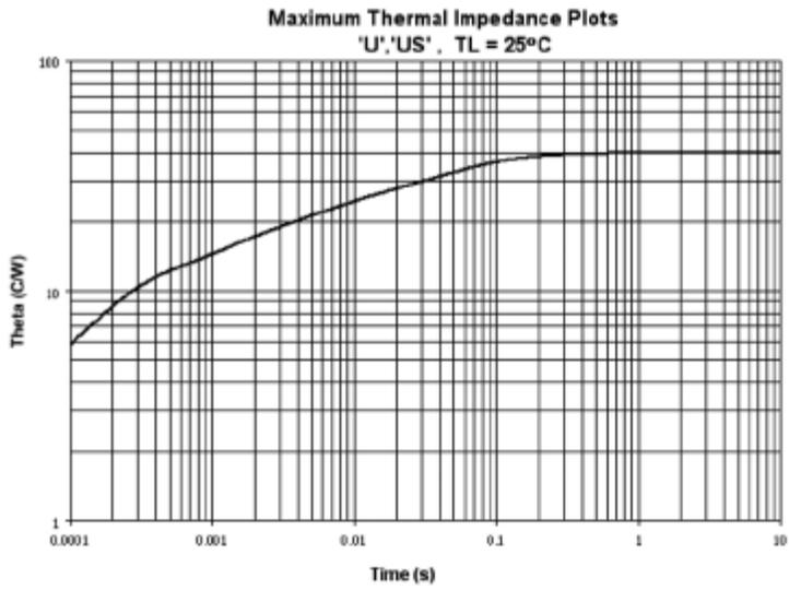
**FIGURE 6.** Thermal impedance – all U and US devices.
