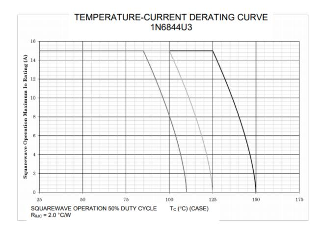
FIGURE 2. Temperature-current derating curve.
