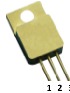
TO – 257 (Isolated Base-plate Hermetic Package)
