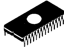
CERAMIC PACKAGE DIP-28C-C01
