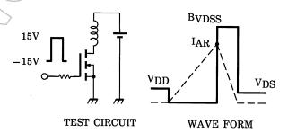
$$\begin{aligned} &R_G = 25 \ \Omega \\ &V_{DD} = 90 \ V, \ L = 22.9 \ mH \end{aligned} \qquad EAS = \frac{1}{2} \cdot L \cdot I^2 \cdot \left( \frac{BVDSS}{BVDSS - V_{DD}} \right)$$
