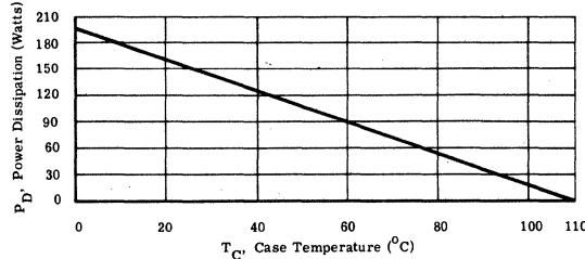
The maximum continuous power is related to maximum junction temperature by the thermal resistance factor.
