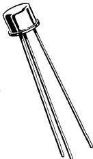
NPN silicon annular transistors designed for high-current, high-frequency amplifier applications.
