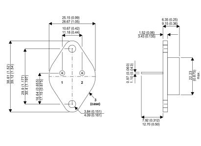
Bipolar PNP Device in a Hermetically sealed TO3 Metal Package.
