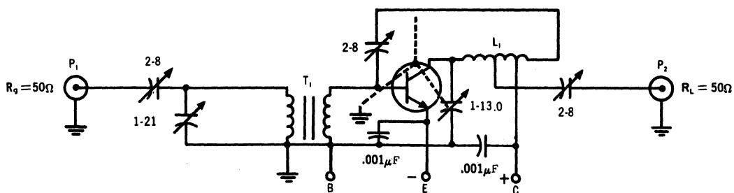
$L_1$ -6 turns of #16 tinned wire; 3/8" ID; Air wound; winding length 3/4";  $\frac{V_C}{C}$  feeds tap 4 1/4 turns from collector end; output tap 3 1/2 turns from collector end.
