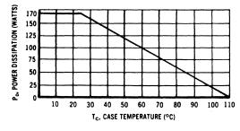
The maximum continuous power is related to maximum junction temperature by the thermal resistance factor. This curve has a value of 170 Watts at case temperatures of  $25^{\circ}$ C and is 0 Watts at  $110^{\circ}$ C with a linear relation between the two temperatures such that:
