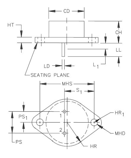
FIGURE 1. Physical dimensions (TO-204AA, formerly TO-3).
