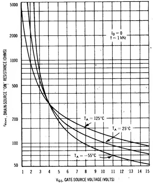
FIGURE 4 — "ON" DRAIN-SOURCE VOLTAGE
