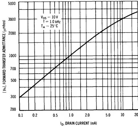
FIGURE 2 — TRANSFER CHARACTERISTICS
