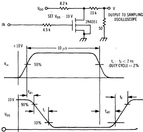
The switching characteristics shown above were measured in a test circuit similar to Figure 10. At the beginning of the switching interval, the gate voltage is at ground and the gate-source
