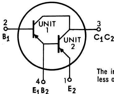
The input unit is identified as Unit 1 regardless of terminal numbering.
