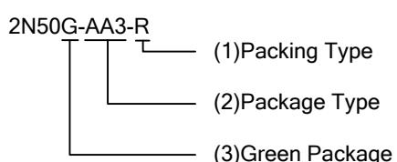
(1) B: Tape Box, K: Bulk, T: Tube, R: Tape Reel
