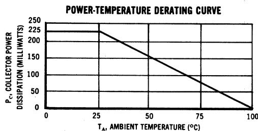
The maximum continuous power is related to maximum junction temperature by the thermal resistance factor.
