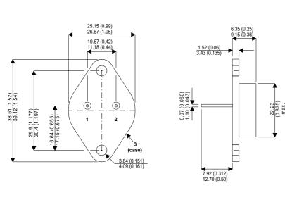
Bipolar NPN Device in a Hermetically sealed TO3 Metal Package.
