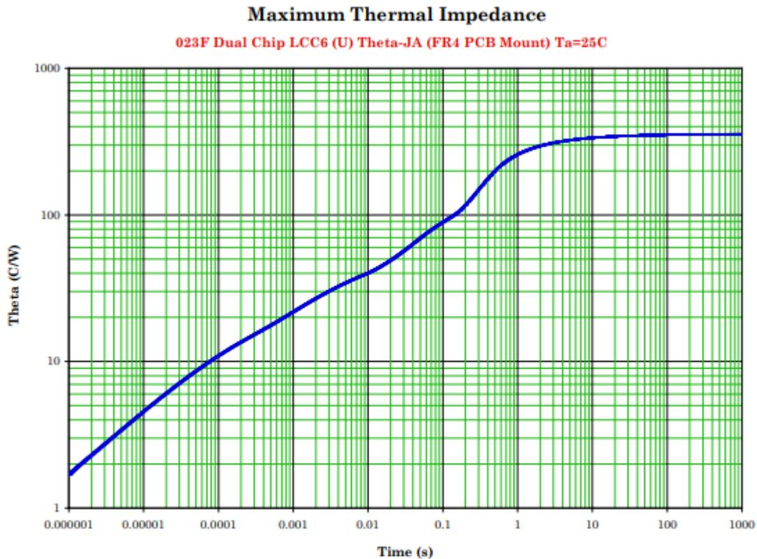
FIGURE 5. Thermal impedance graph ( $R_{\theta JPCB}$ ) for 2N5794U, 2N5794UC, 2N5794AU, and 2N5794AUC (U and UC).
