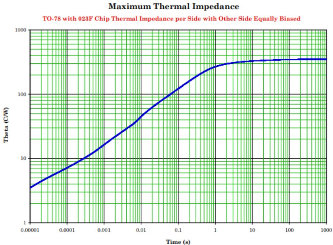
FIGURE 6. Thermal impedance graph ( $R_{\theta JA}$ ) for 2N5794U, 2N5794UC, 2N5794AU, and 2N5794AUC (U and UC).
