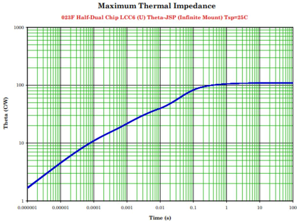
FIGURE 4. Thermal impedance graph ( $R_{\theta JSP}$ ) for 2N5794U, 2N5794UC, 2N5794AU, and 2N5794AUC (U and UC).
