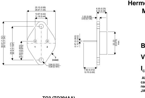
Bipolar NPN Device in a Hermetically sealed TO3 Metal Package.
