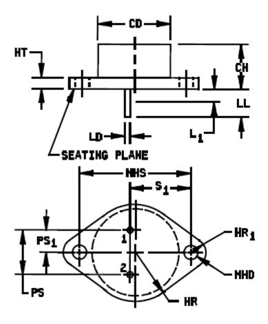
FIGURE 1. Physical dimensions (similar to TO-204AA formally TO-3).
