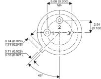
**PINOUTS**1 – Source 2 – Gate 3 - Drain
