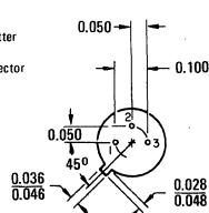
Collector Connected to Case
