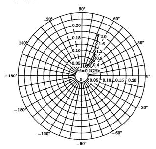
$\begin{array}{c} S_{22e} \\ V_{CE} = 8V \\ I_{C} = 5mA \\ T_{a} = 25^{\circ}C \\ (UNIT: \Omega) \end{array}$
