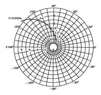
$S_{12e}$   $V_{CE}=8V$   $I_{C}=5mA$   $T_{a}=25^{\circ}C$
