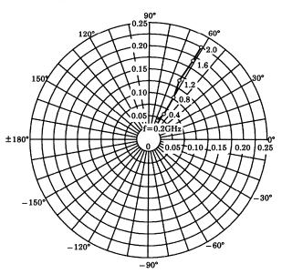
$\begin{array}{l} S_{22e} \\ V_{CE} = 8V \\ I_{C} = 5mA \\ Ta = 25^{\circ}C \\ (UNIT:\Omega) \end{array}$
