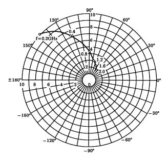
$S_{12e}$   $V_{CE} = 8V$   $I_{C} = 5mA$  $T_{a} = 25^{\circ}C$
