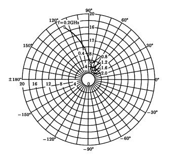
$\begin{array}{l} S_{12e} \\ V_{CE} = 8V \\ I_{C} = 20 \text{mA} \\ Ta = 25^{\circ}C \end{array}$
