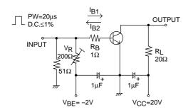
IC=10IB<sub>1</sub>= -10IB<sub>2</sub>=1A (For PNP, the polarity is reversed.)
