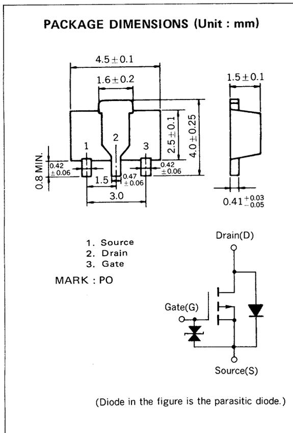
The 2SJ212, P-channel vertical type MOS FET, is a switching device which can be driven directly by the output of ICs having a 5 V power source.
