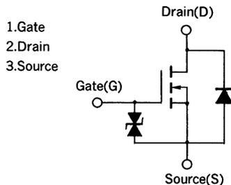
(Diode in the figure is the parasitic diode.)
