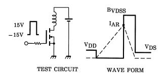
$$\begin{split} R_G &= 25~\Omega \\ V_{DD} &= 50~V,~L = 3.3~mH \end{split}$$
