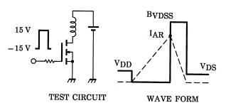
$$\begin{aligned} &RG = 25~\Omega \\ &V_{DD} = 50~V,~L = 56.7~mH \end{aligned} \qquad E_{AS} = \frac{1}{2} \cdot L \cdot I^2 \cdot \left( \frac{BV_{DSS}}{BV_{DSS} - V_{DD}} \right)$$
