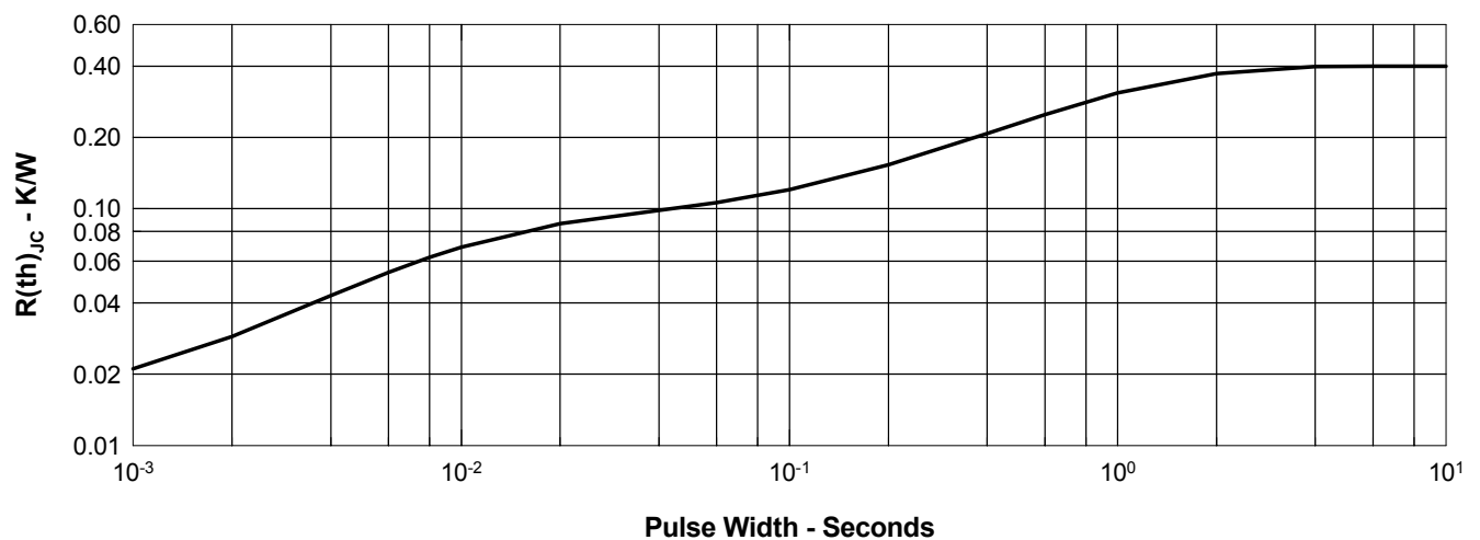
Figure 10. Transient Thermal Resistance
