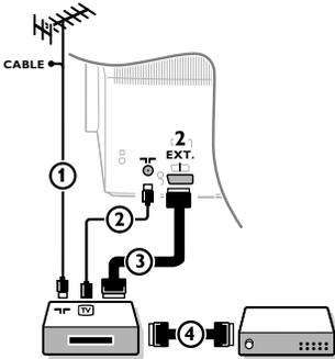
Connect the aerial cables ①, ② and, to obtain the optimum picture quality, eurocable ③ as shown.
