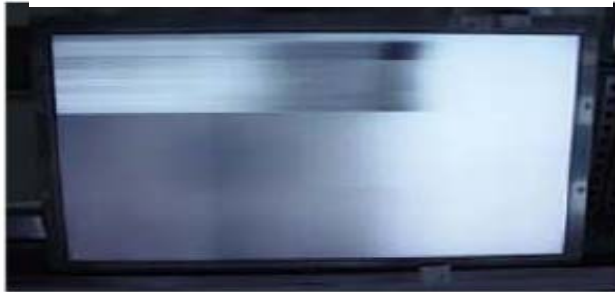
Horizontal Block Gate TAB IC Defect
