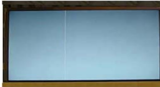
Vertical Line Source TAB IC Defect
