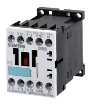
CONTACTOR, AC-3 3 KW/400 V, 1 NO, AC 230 V, 50/60 HZ, 3-POLE, SIZE S00, SCREW CONNECTION
