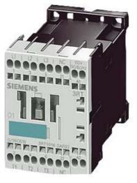
CONTACTOR, AC-3 3 KW/400 V, 1 NO, AC 230 V, 50/60 HZ, 3-POLE, SIZE S00, CAGE CLAMP CONNECTION
