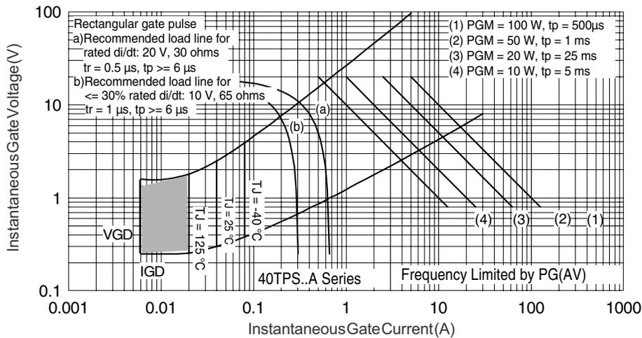
Fig. 8 - Gate Characteristics
