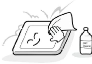
4. Leaving water or other fluids on the panel screen for an extended period of time can result in discoloration or stripes. Immediately remove any type of fluid from the screen.
