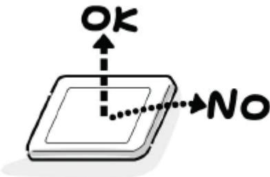
2. Carefully align the holes at all four corners of the LCD module with the corresponding holes in the LCD cover and fasten with screws. Do not strongly push on the module
