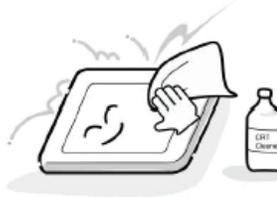
5. Leaving water or other fluids on the panel for an extended period of time can result in discoloration or stripes. Immediately remove any type of fluid from the screen.
