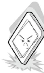
7. CMOS-LSI circuitry is used in the LCD module, so avoid damage due to static electricity. When handling the module, use a wrist ground or anchor ground.
