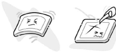
4. If the panel surface becomes soiled, wipe with cotton or a soft cloth. If this does not remove the soiling, breathe on the surface and then wipe again. If the panel surface is extremely soiled, wipe the panel surface with CRT cleaner sprayed onto the cloth. Do not spray the cleaner on the panel. Pay attention not to scratch the panel surface.
